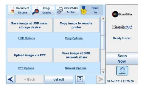
Scanner users simply press a button to save their images to a connected USB device and scan. Once they have scanned their documents, they can check the files stored on their USB device by selecting the link <u>USB Options</u>. This displays a list of files contained on their device, letting users check to ensure that all files are stored.
