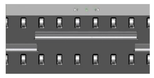
The reason for these stitching problems is the staggered orientation of the individual CIS lines which have a typical distance of about 25mm or one inch. If the document speed changes between these two positions, the CIS element will not exactly scan the same line, producing a visible vertical shift at the position where the CIS modules mate. The transport drums are all actively driven by the main motor to
